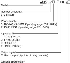
Optional specification Blank: With socket /SN: Without socket
