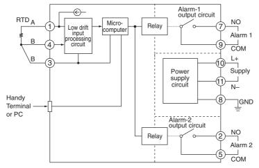
Note: Make the wiring resistance of the input terminals 1 and 3 the same.
